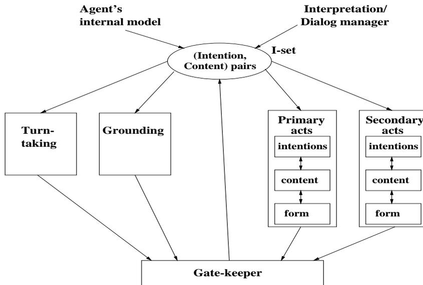
Figure 4: Proposed generator architecture
