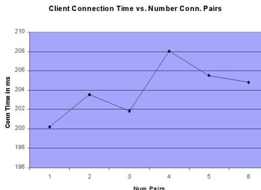
Figure 1: Connection times for the KDC protocol
