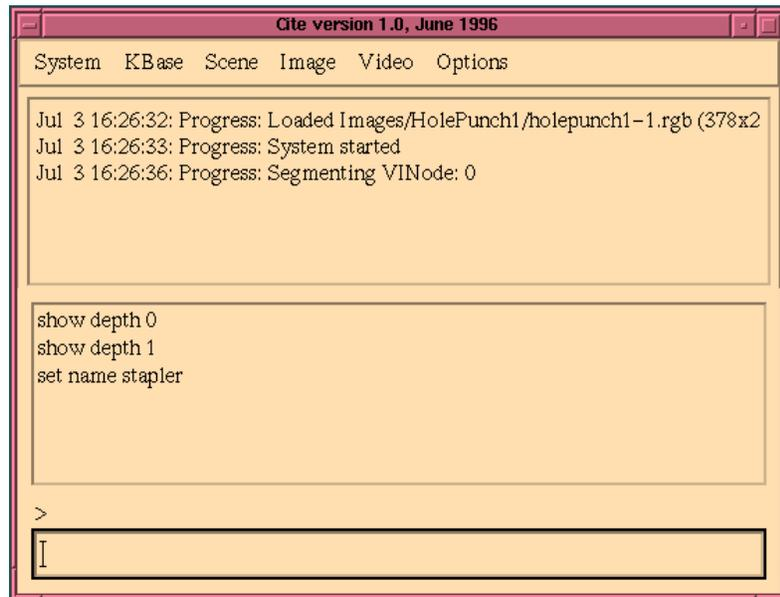
command prompt. Figure 28 shows the command window as it normally appears. The top text window contains the status and progress-reporting messages from CITE. The middle text window is a history of the previous entered commands, and the lower text window is the command prompt.
