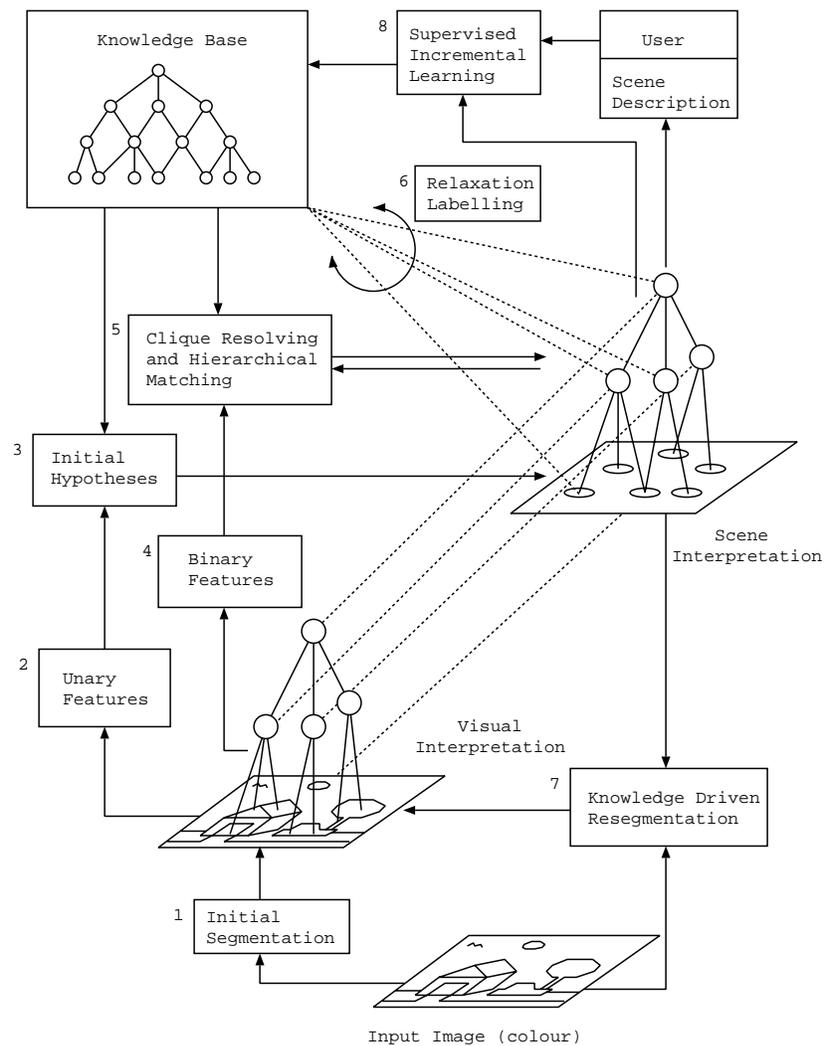
one with, in principal, no depth limitation. Multiple hypotheses are generated for each scene element, and these are resolved using a hierarchical extension to relaxation labeling.
