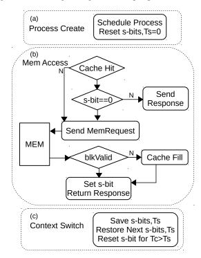
process creation, execution, and preemption/resumption at the time of a context switch. Software saves and restores the *s*-*bits* for a process executing on a hardware context to/from memory at the time of a context switch. Additionally, software maintains Ts for each process, which is the time the process was most recently preempted. A newly created process has both Ts and *s*-*bits* reset when it is scheduled for the first time.
