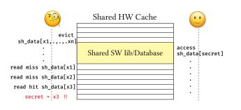
Fig. 2: Reuse attack in cache
