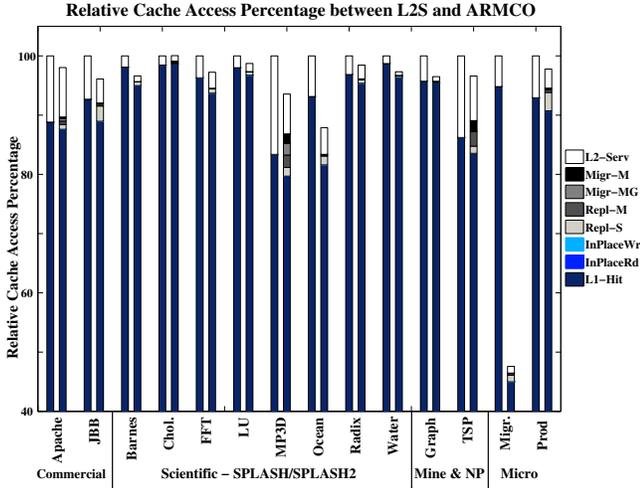
**Figure 5.** Normalized cache access distribution (16 threads). InPlaceRd and InPlaceWr occur at the predicted L1 cache without cache line allocation at the requester L1. Rep-S and Rep-M refer to remote L1 hits resulting in replication via L1-to-L1 transfers where the cache line is in shared and modified state respectively. Migr-M and Migr-MG refer to remote L1 hits resulting in migration via L1-to-L1 transfers where the remote cache line is in modified and migratory state respectively.
