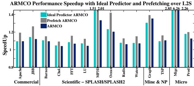
**Figure 9.** Normalized Performance of ARMCO with ideal prediction, ARMCO with ideal prediction and prefetch, and ARMCO with regular predictor over L2S (16 threads). Prefetching effect is incorporated by zero-latency fetching at request time from predicted L1 if the requested data line is at stable state in the system
