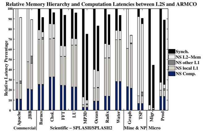
**Figure 4.** Timing breakdown among computation, different levels of the memory hierarchy, and synchronization, normalized to L2S (16 threads). For commercial workloads, we do not distinguish between synchronization and non-synchronization time. ‘Synch’ is all synchronization time spent in both computation and the memory hierarchy. ‘NS’ refers to non-synchronization. ‘other L1’ refers to time spent in direct L1-to-L1 transfers.
