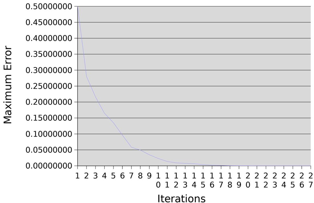
This instance of our Value Iteration program was set to converge on utility estimates until it was below an error threshold of  $1/1,000,000$ . The algorithm converges to good estimates quickly, but takes a long time to converge to extremely accurate utility estimates.
