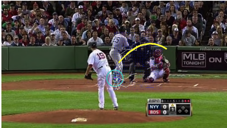
Figure 1: The final frame of a video. Moving points are in teal, clusters marked with a teal circles. Motion paths are drawn in white, and the path of the ball is identified in yellow.
