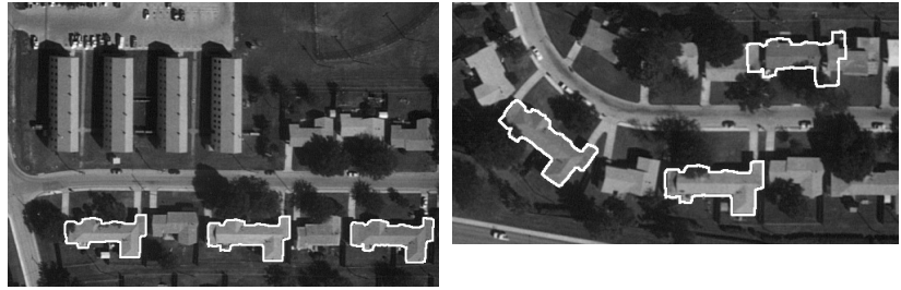
Figure 7. Duplexes extracted from two images. In the image on the left, all three duplexes were correctly identified. On the right image, a false positive appears on the upper right side. The half-visible duplex to the bottom right is the only false negative encountered during testing.
